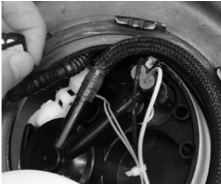
5. Rotate the unit to ensure the vent valve is positioned between two of the side retainers (not on top)
