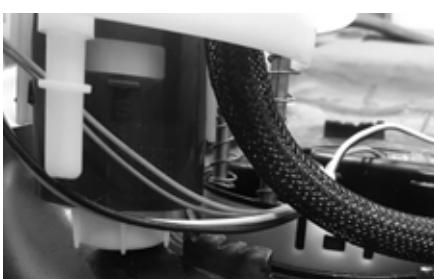
6. Slide the module at an angle through the opening, Slide the module in sideways a little
